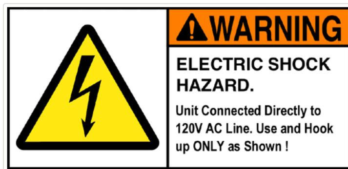
The circuit is connected directly to the high voltage (120VAC) AC line so care must be taken when handling this circuit. It should ultimately be inside a proper enclosure to prevent it from being a shock and fire hazard.
